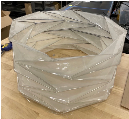
Origami Solar Panel Bellow (6 meter deployed diameter) [PATENT PENDING]
